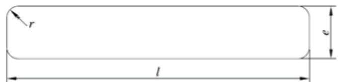
Profile C: Flat bar with straight edges and rounded corners
