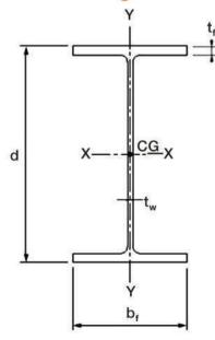
The masses of sections with at least one dimension greater than 76 mm may not vary by more than 2.5% of the specified theoretical mass, except for sections weighing less than 150 kg/m, where the variation must be between -2.5% and +3.0% of the specified theoretical mass.
